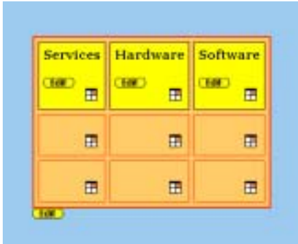
Figure 10: A table in edit view. The Edit tag on the bottom opens the Table Layout Properties tool; the three edit tags in the top row open the Edit Text / Links / Small Tables tool; and the nine four-square icons open the Edit Table Cell Properties tool.
